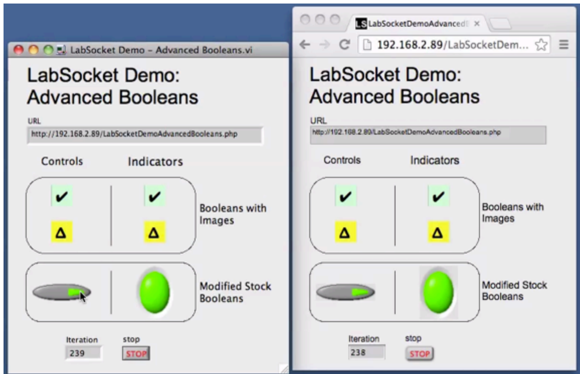
Figure 8.3. Screenshot demonstrating high-fidelity representation of Boolean elements (L- LabVIEW VI, R – Browser)
